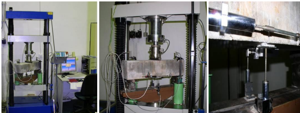
Figure 1.: Testing apparatus – a) loading apparatus, b) testing specimen, c) detail of measuring sensors.
